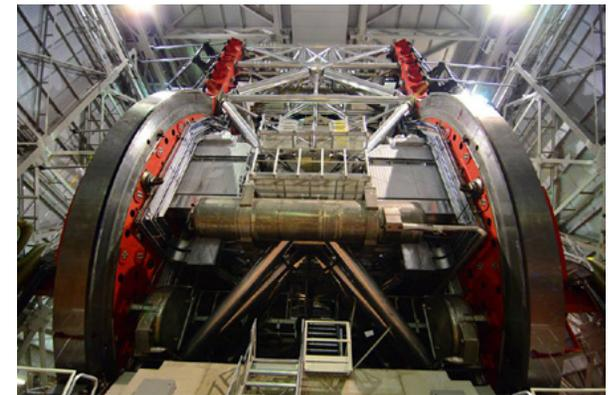
The Large Binocular Telescope uses two 8.4-meter mirrors supported by a massive structure. [Wayne Schlingman]
