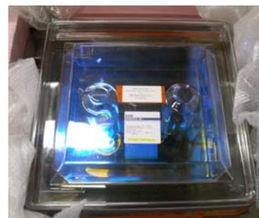
Figure 3: ODI r'-band filter in its shipping container. It is 42cm x 42cm.
