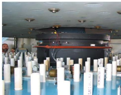
Figure 2: Primary being lowered onto the mirror cell.
