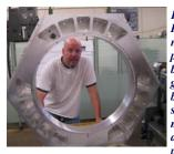
Figure 1: Instrument maker, Ron Harris, standing behind the aluminum Atmospheric Dispersion Compensator (ADC) housing (Part Number ODI-ME-02-1037). Three triangular shaped outrigger blocks will bolt to the housing to form the main structural component to which filter mechanisms and axles, ADC cells, and dewar will mount. When complete the housing will weigh 170 lbs
