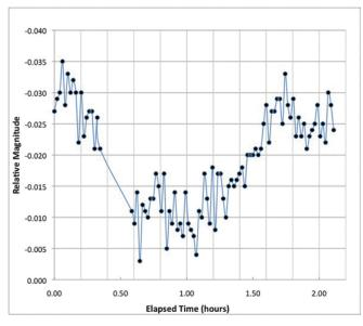
Figure 3: Lightcurve of the transiting, hot-Jupiter planet TrES-2b obtained at the Kitt Peak Visitor Center 0.5-m telescope in a z-band filter. The data gap from 0.3-0.6 hours was caused by repositioning of the telescope at meridian crossing.
