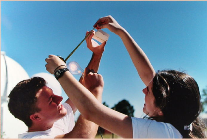
Students measuring the Sun's luminosity with a wax cube and a light bulb.
