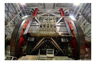
The Large Binocular Telescope uses two 8.4-meter mirrors supported by a massive structure. [Wayne Schlingman]
